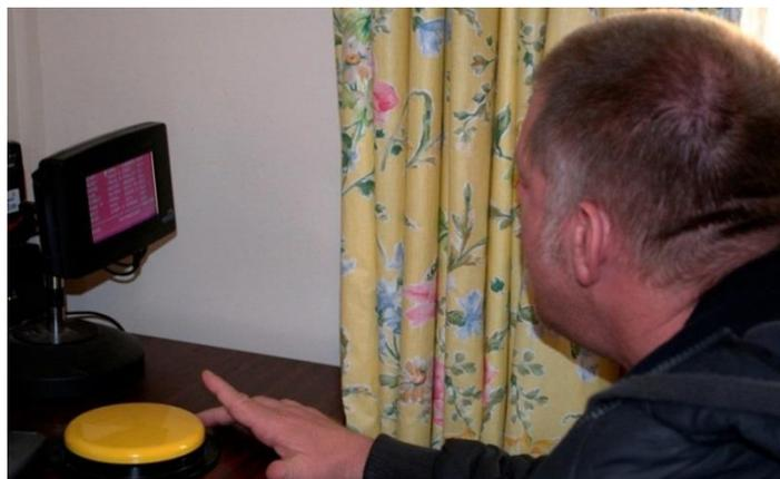
I use a Possum system to control my phone, front door, call system and various electrical devices which enable me to live independently.
